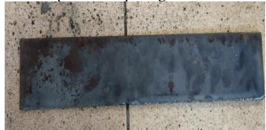
Gambar 2. Logam ST37 Dengan Dimensi (50x3x450mm)
