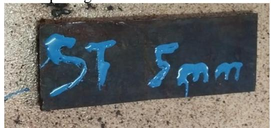
Gambar 3. Logam ST37 Dengan Dimensi (50x5x200mm)
