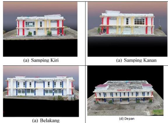
Gambar 9 Hasil Mesh dan Texture dari pengolahan dense point cloud Pix4d Mapper (a) Samping Kiri, (b) Samping Kanan, (c) Belakang (Sumber: Pengolahan Data 2024)
