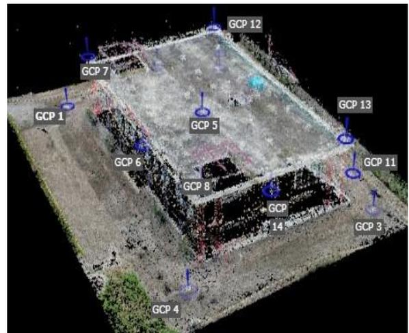
Gambar 5. Hasil Point Cloud Pix4d Mapper (Sumber : Pengolahan Data 2024)
