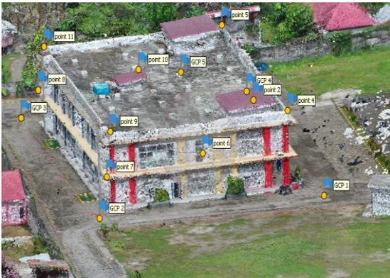
Gambar 6. Hasil Dense Point Cloud Agisoft Photoscan (Sumber : Pengolahan Data 2024)
