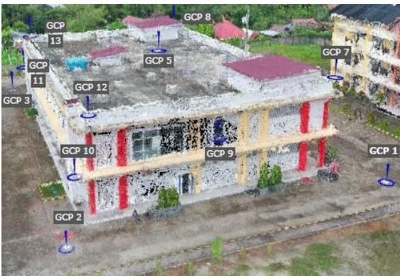
Gambar 7. Hasil Dense Point Cloud Pix4d Mapper (Sumber : Pengolahan Data 2024)
